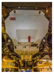
Made from pressed and folded 3mm steel, ARB's underbody protection plates are designed to shield the vehicle's steering, sump, gearbox and transfer case from impacts on rocks and tree stumps. They help keep it moving off-road, too, by providing a smooth surface capable of sliding over obstacles - particularly useful on long-wheelbase vehicles like double-cabs. Secured to the chassis, the plates are removable for servicing, but that's about all they'll shift for
